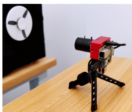
Fig. 9. Prototype of EV-Tach on Raspberry Pi 4B
