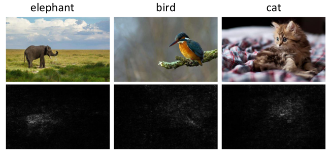
Fig. 4. Back-Propagation-Guided interpretation (BPGI). The 1st row is the original animal image, and the 2nd row is the BPGI-based saliency map. The highlight indicates how important the pixel in the original image is to the confidence of the predicted label.
